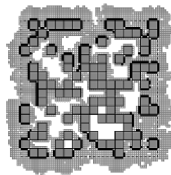
Fig. 3. Final stage of Nafion filling the support grain pores. The amount of Nafion particles that can be located on the surface of carbon black particles forming the support grain is 854, the amount of Nafion active particles is 401, platinum utilization degree \psi = 0.47 . The amount of particles that can be located along the support grain perimeter is 4 \times 16 \times 4 = 256 , "diffuseness" factor of the contact surface of the ionic and gas percolation clusters \xi = 1.57 . \nu = 0.62 , L/d = 16 , d/d_n = 4 , p_s = 1 , p_n = 0.001 , particle free path = 16.
