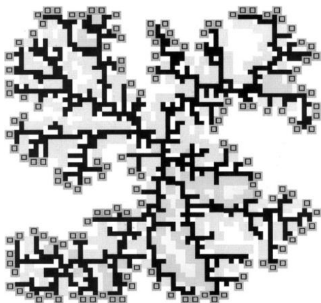
Fig. 5. Distribution of enzyme molecules (a square of conventional size of 1 \times 1 designated by gray squares with a black frame inside) at a random fractal cluster of carrier particles (a square with the size of 2 \times 2 marked black) with the size of 61 \times 61 . All the sites at the cluster perimeter that can potentially be filled by the enzyme molecules are marked gray. The amount of the carrier particles is 908, the number of the enzyme molecules immobilized at the cluster is 146, the number of all the sites at the cluster perimeter accessible for the enzyme molecules is 374. The fractal dimension of the cluster D = 1.6 .
